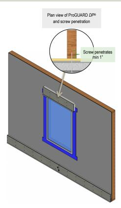
Ensure screw length selected allows for a minimum of 1" penetration into the stud structural back-up behind the sheathing. Calculation for minimum screw length:
