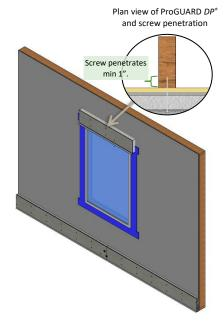
Ensure screw length selected allows for a minimum of 1" penetration into the stud structural back-up behind the sheathing. Calculation for minimum screw length:
