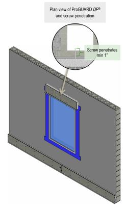
Ensure screw length selected allows for a minimum of 1" penetration into the concrete structural back-up. Calculation for minimum screw length:
