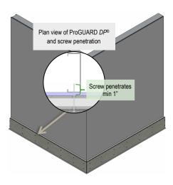
Ensure screw length selected allows for a minimum of 1" penetration into the stud structural back-up behind the sheathing. Calculation for minimum screw length:
