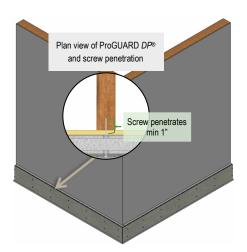
Ensure screw length selected allows for a minimum of 1" penetration into the stud structural back-up behind the sheathing. Calculation for minimum screw length:
