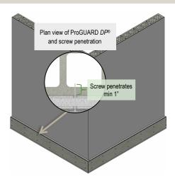
Ensure screw length selected allows for a minimum of 1" penetration into the concrete structural back-up. Calculation for minimum screw length:
