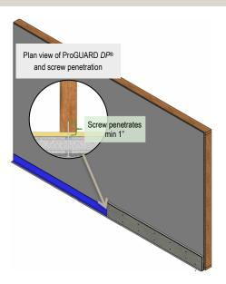
Ensure screw length selected allows for a minimum of 1" penetration into the stud structural back-up behind the sheathing. Calculation for minimum screw length:
