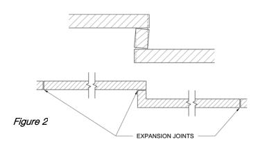
Wall Openings: More movement will tend to occur above and below openings due to the change in the wall's mass. The differential movement between areas of different wall mass may cause cracks to emanate from the corners of the openings. As these openings also tend to "weaken" the wall, they act as naturally occurring movement joints.
