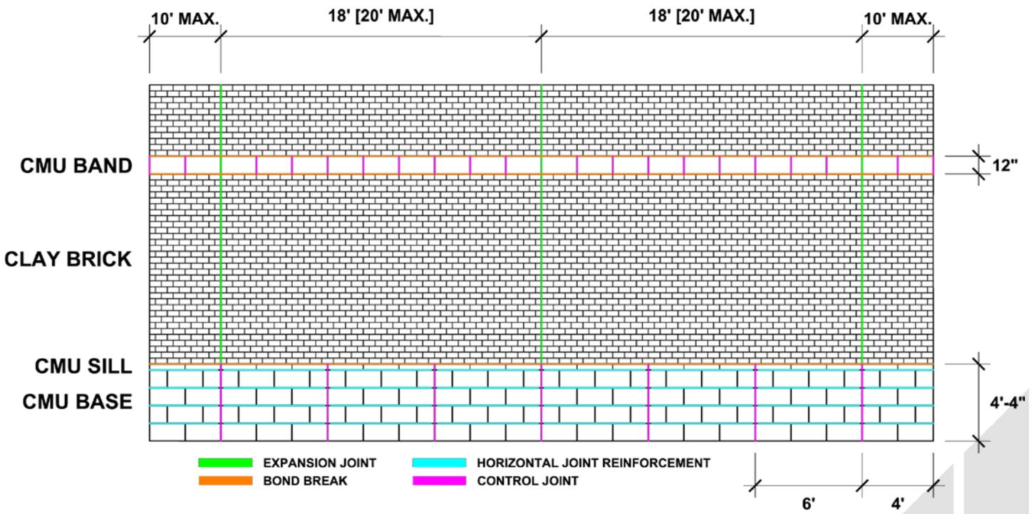
Note that the horizontal joint reinforcement in the beds of the concrete masonry units should not bridge the control joints.
