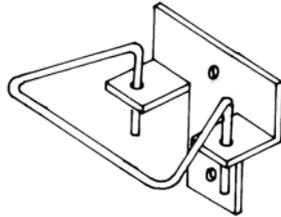
Some examples of adjustable tie types include pintles, slotted, and fastener adjusted.
